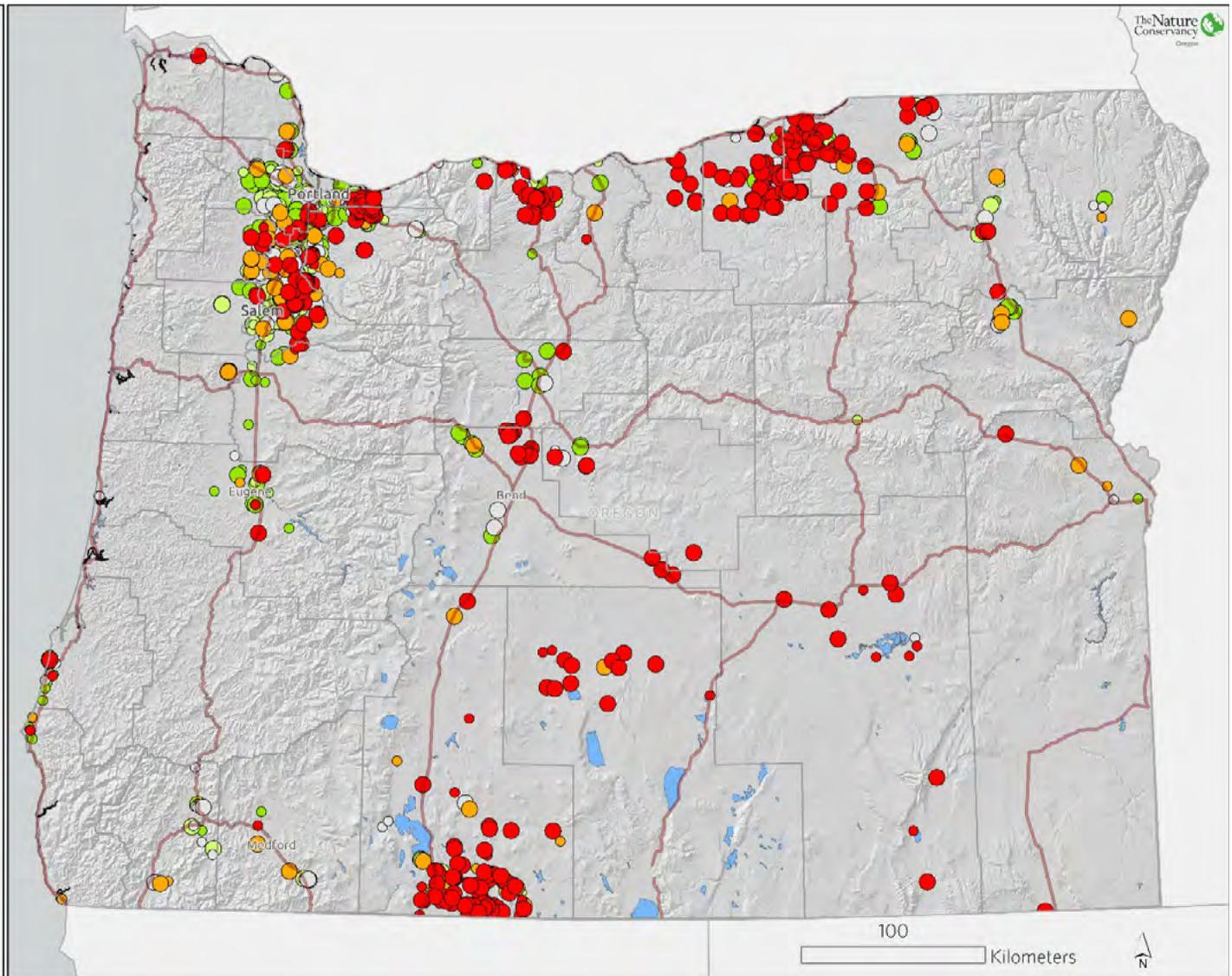
**Figure B1 i b:** Groundwater withdrawals: observed monitoring well declines with a fifteen-year period of record
