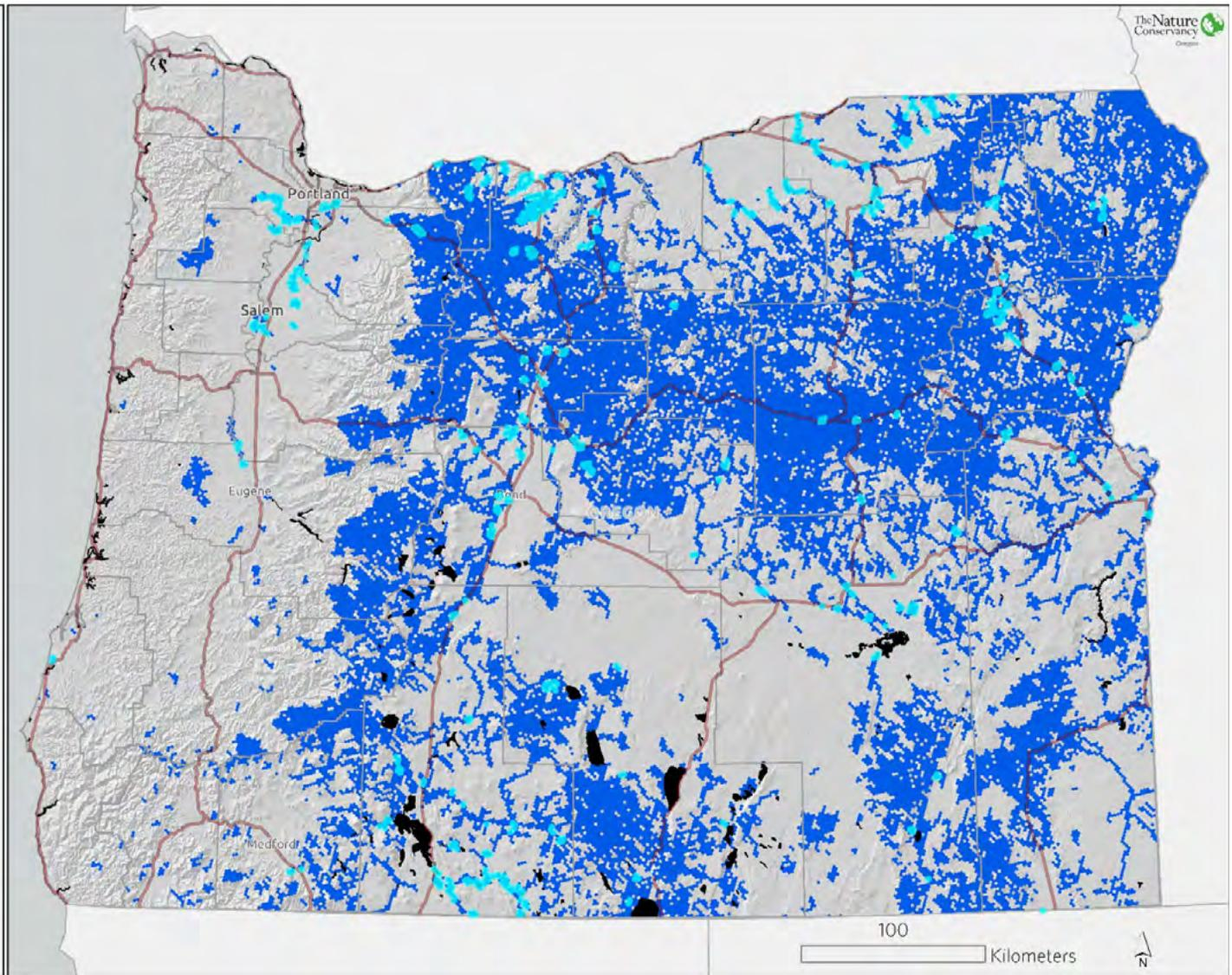
**Figure B2 i h:** Groundwater withdrawals: groundwater-dependent rivers near monitoring wells
